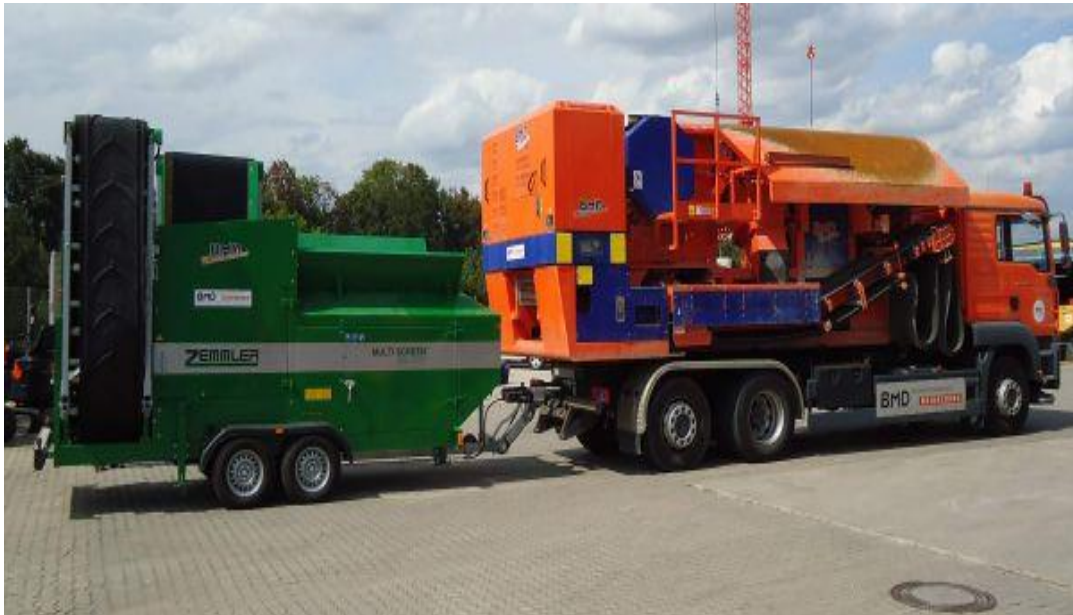
Figure 4 - Mobile Building Waste Recycling Plant with granulator (mobile sieve)
