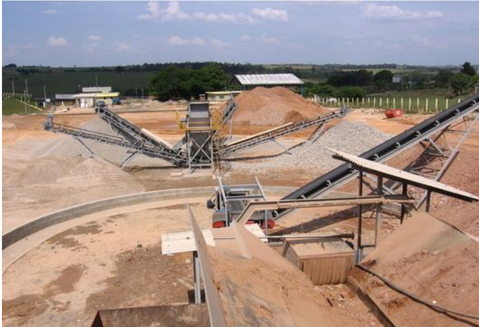
Figure 3 - Fixed Recycling Plant for Civil Construction Solid Waste
